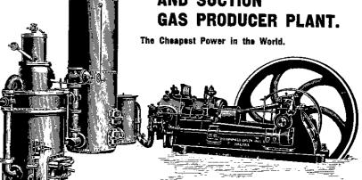
A 25-b.h.p. at Wanganui works on 11/4lbs of coke per horse-power per hour. A 40-b.h.p., installed for Messrs. Lind & O'Connor, Flaxmillers, Shannon, is now at work. All interested are invited to inspect.
