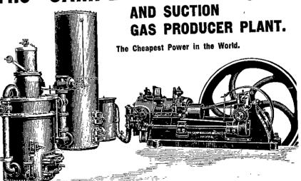
A 25-b.h.p. at Wanganui works on 111bs of coke per horse-power per hour. A 40-b.h.p., installed for Messrs. Lind & O'Connor, Flaxmillers, Shannon, is now at work. All interested are invited to inspect.
