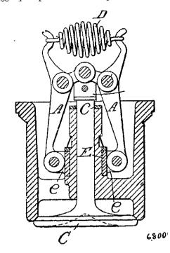
and controlled by a spring (d). The advantage of this valve is that it requires a greater degree of suction to first open it than it does to maintain it open, whereas the reverse is the case with ordinary suction valves, so that these latter are often uncertain in action owing to their "fluttering."
