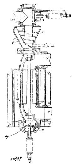
cone-shaped member (a). In the spiral passage (d) the heavier parts of the fuel are discharged by centrifugal action, whilst the lighter and properly carburetted portion passes on by the outlet (n) and conduit (u) to the cylinder of the engine. Additional air may be admitted by the valve (s).
