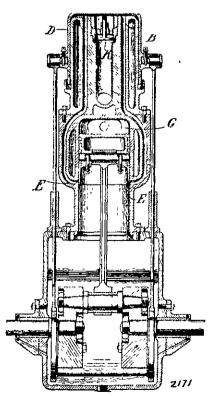
its working stroke, the cylinder (d) is raised so that a vacuum is formed therein. When the piston (f) passes the ports (e) in its cylinder, the exhaust gases escape through these to the cylinder (d),
