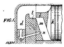
of the cylinder, so that, as the piston arrives at the end of its stroke, it super-compresses a charge in the chamber (m). This super-compressed charge escapes by the passage (n), where it meets the fuel, which it atomises as it is discharged from the outlet (d). The same invention can be applied
