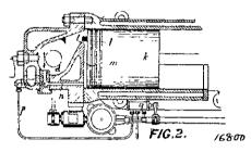
to four-stroke-cycle engines, as shown in Fig. 2, where a web (l) is secured to the piston and cooperates with a fixed part at the combustion end of the cylinder to form a separate chamber (m), in which super-compression takes place at the end of the stroke. In this figure fuel is shown as admitted by the conduit (p).
