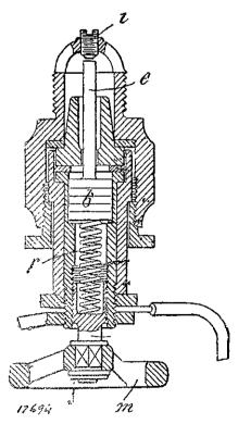
that when the required degree of compression is obtained within the cylinder the piston (b) is forced back thereby, and thus the circuit  $(e \ i)$  is broken so that a spark occurs. By regulating the pressure exerted by the spring (r), adjustable by the hand wheel (m), the moment of ignition can be controlled.
