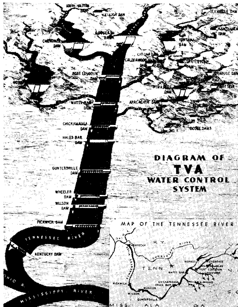
DIAGRAM of the Tennessee Valley Authority water control system
