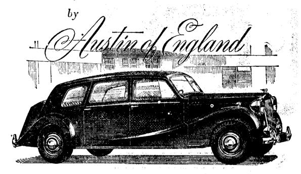
THE AUSTIN "A125" SHEERLINE TOURING LIMOUSINE ... is a powerful eight-seater car, distinguished in appearance and luxuriously equipped. Its smooth, silent road performance and the tasteful design of its interior furnishing induce a sense of well-being and provide exceptional comfort. The many notable chassis features of this fine car include a six-cylinder overhead-valve engine of 4-litre capacity, independent front suspension, steering column gear change control and a hypoid rear axle.
