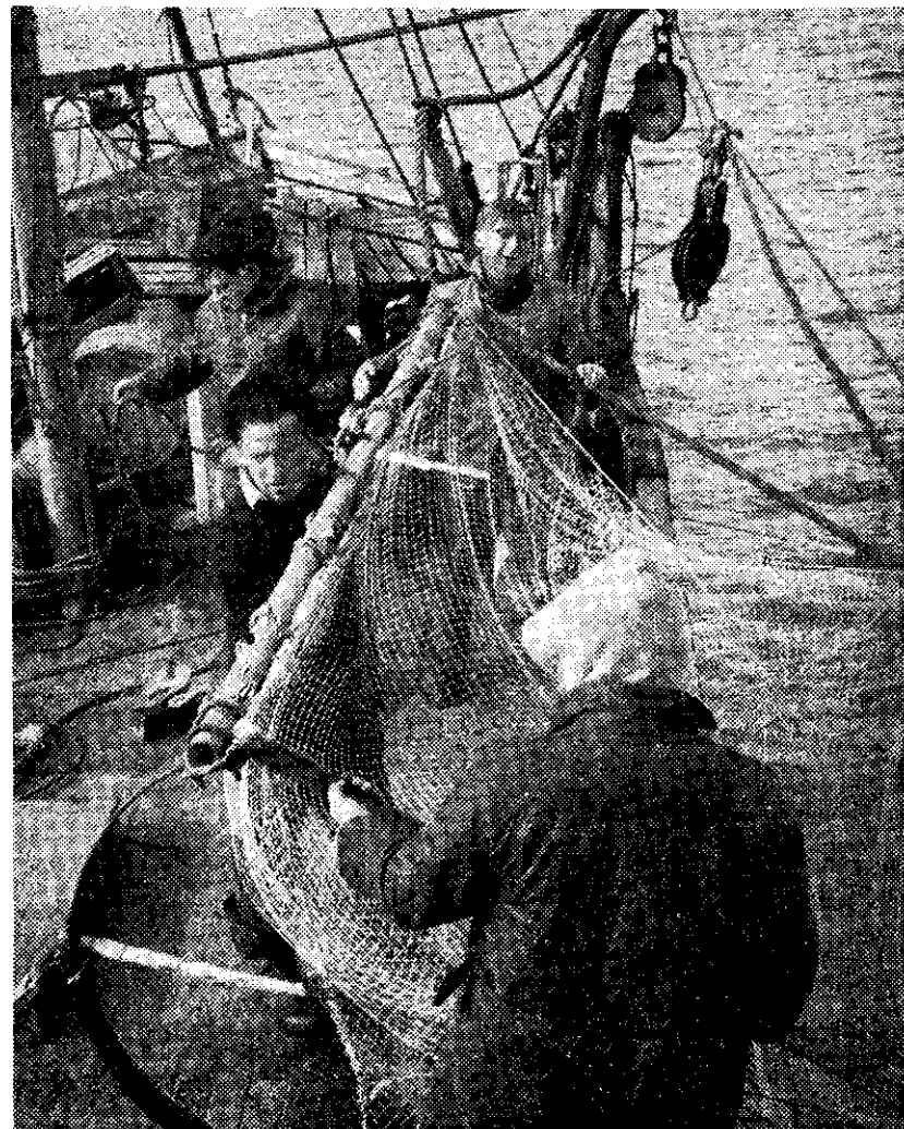
PREPARING to send down the beam trawl: Scientists at work aboard the Admiral
