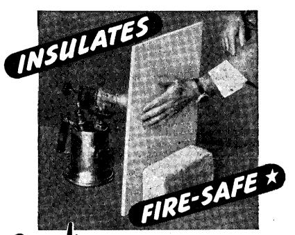
A blow lamp after five minutes barely warmed the other side of a sheet of Gibraltar Board . . . the wallboard which shuts out heat and cold, quietens noise, and, with a gypsum-pumice core which WON'T BURN.
