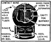
cable spaced to the desired length before the mine is put into the water. When the sinker reaches the sea-bed, the force of impact releases an automatic device which pays out sufficient cable to allow the mine to rise until it is held beneath the surface of the water.
