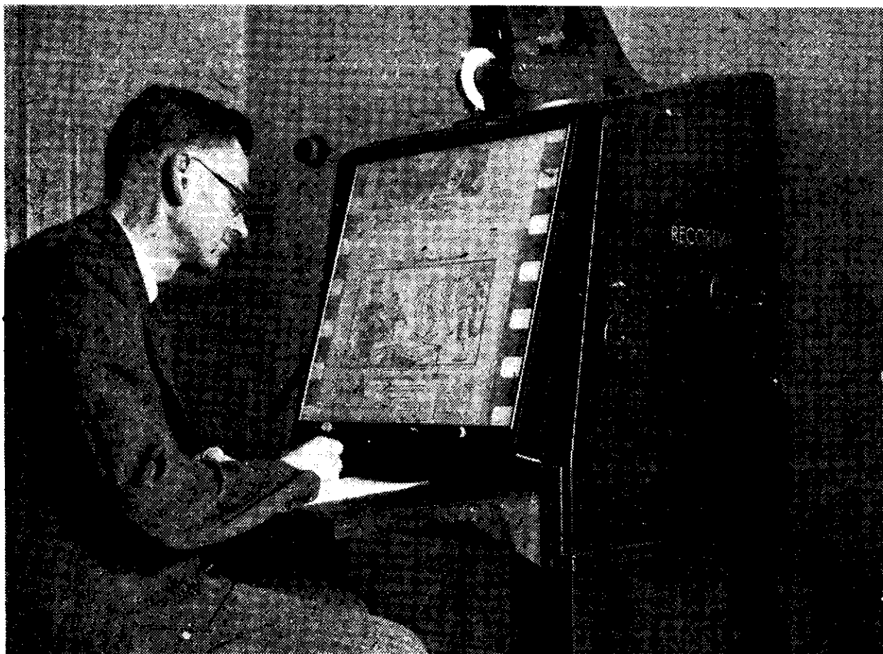
USING a microfilm "reader." The film runs across the top of the apparatus and the screen image is in most cases larger than the original
