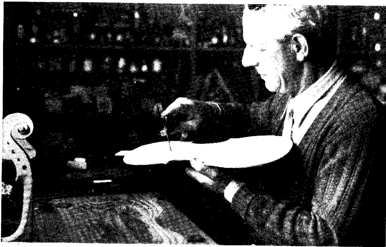
Left: ERIC MEIER tests the thickness of the wood in a violin "belly," using a specially-designed gauge
