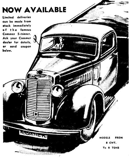
The Commer 5-ton "Superpoise" model has a 6-cylinder engine, heavy duty dry plate clutch, robust 4-speed gearbox with constant mesh helical gears, heavy ribbed cast steel rear axle, rugged frame, all-steel cab, hydraulic brakes, etc. Designed throughout to perform heavy-duty work with economy and reliability. Chassis supplied complete with "Diaflex" mounted cab which is insulated from distortion.
