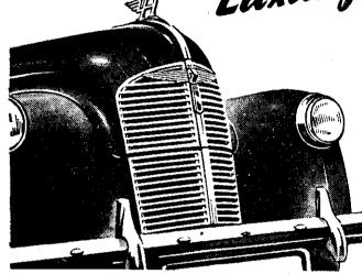
Powerful 4-cylinder overhead-valve engine, developing 40 b.h.p. • Independent front-wheel suspension • Girling hydro-mechanical brakes with pistol-grip hand-brake • All four doors rear-opening for safety and convenience • Bonnet lock controlled from inside car • Concealed door-hinges and built-in running boards • Latest type, easy-clean wheels • All-steel, sound insulated
