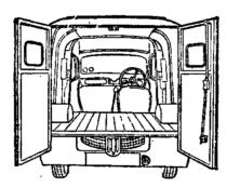
Body is of steel, with board floor and strongly hinged rear doors. Note the wide-opening doors and unobstructed loading space.
