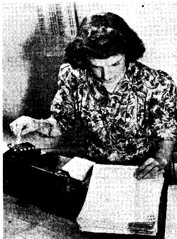
—AND IT COMES OUT HERE: Left—Records of interviews in the Survey of Listening being punched on cards for subsequent tabulation. Right—Electrical counter-sorter in operation. This machine counts the number of times each broadcast has been heard by the persons interviewed
