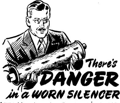
A very real danger-because when a silencer is rusted through and full of holes, the exhaust fumes, containing deadly carbon monoxide gas, are liable to seep into your car, and cause a serious accident—even death. Old cloggedup silencers restrict the flow of exhaust gases, affecting engine efficiency and robbing you of precious mileage. What you should do is drive to your nearest garage and have one of the new "Ace" Silencers fitted.
