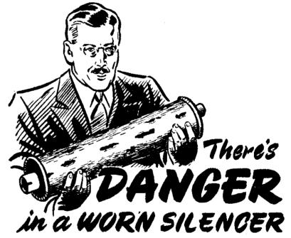
A very real danger-because when a silencer is rusted through and full of holes, the exhaust fumes, containing deadly carbon monoxide gas, are liable to seep into your car, and cause a serious accident—even death. Old cloggedup silencers restrict the flow of exhaust gases, affecting engine efficiency and robbing you of precious mileage. What you should do is drive to your nearest garage and have one of the new "Ace" Silencers fitted.
