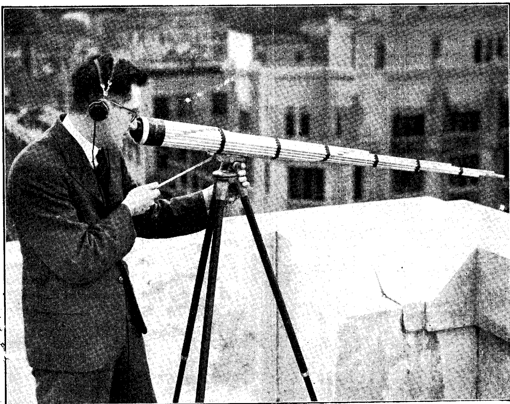
R. E. GRAINGER, Chief Engineer of the Commercial Broadcasting Service, demonstrates the new "machine gun" microphone recently secured for the ZB Stations. (See article on page 53)
