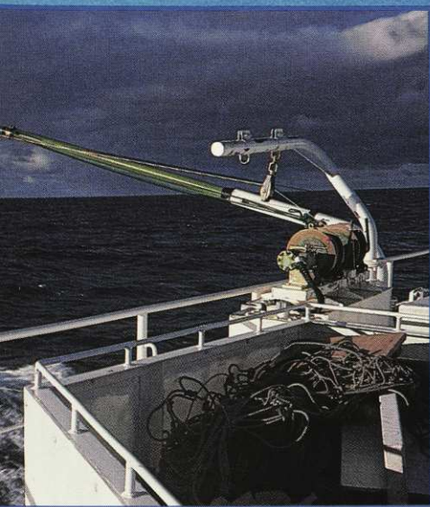
Pole at stern of longline boat. Streamers from this pole scare birds away and can reduce bait loss to birds by 69 percent. Photo: Nigel Brothers.
