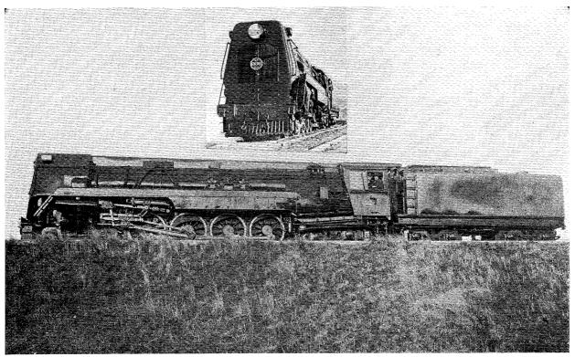
Above: Ka Class Locomotive, 4-8-4 Type. Length Overall, 69 ft. 8 in.; Cylinders, 20 in. by 26 in.; Driving-wheels, 4 ft. 6 in. Diameter; Tractive Force, 30,815 lb.; Weight, 142 Tons.
