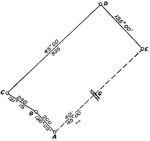
4. From data given, compute the area of the figure ABCD (by any method except scaling or planimeter).
