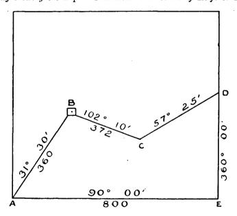
The above diagram represents a mining claim: B the position of a shaft 80 ft. deep, and BCD an underground drive from the shaft to the eastern boundary of the claim, having a fall of 4 ft. 10 in. Distances in links.
