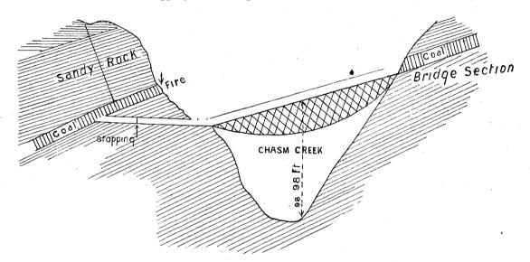
Near 3 on tracing, the fire at outcrop is very fierce; it is at an elevation beyond the effective power of available water.
