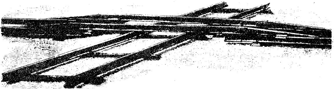
Fig. 81. Bridge Crossing for wheels with one and two flanges.
