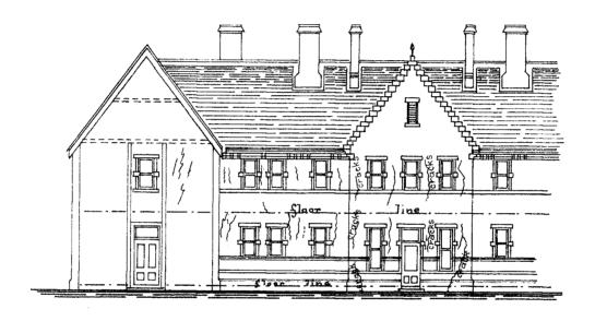
BACK ELEVATION -- SKETCH SHEWING CRACKS THAT OCCURRED IN 1884.
