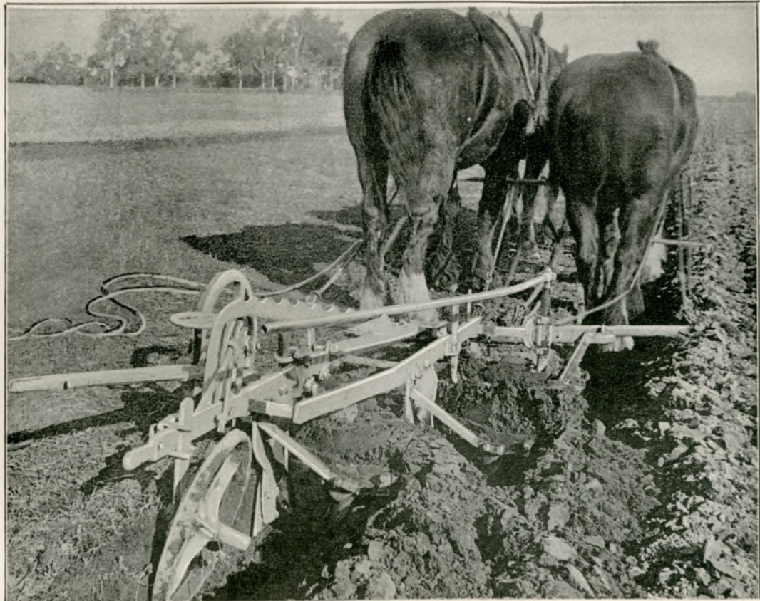
11.V.—HOWARD'S TWO-FURROW DIGGING PLOUGH AND FOUR HORSES AT LINCOLN AGRICULTURAL COLLEGE, NEW ZEALAND.
