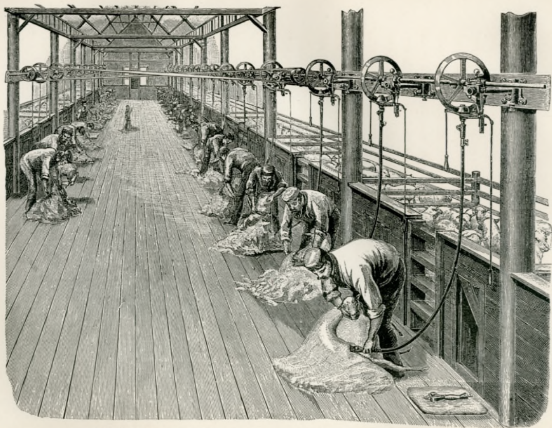
LXXIV.—WOLSELEY SHEARING MACHINE AT WORK IN A WOOL-SHED.
